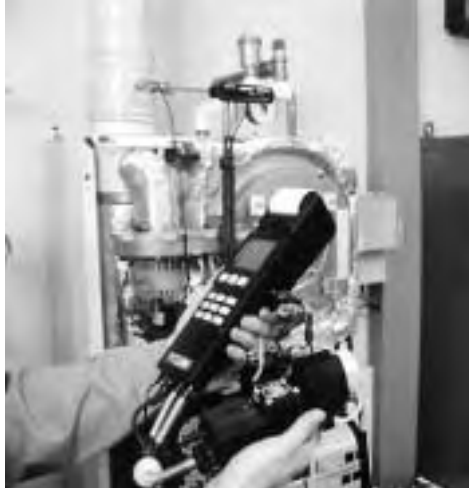
Fig. 24: The gas drier guarantees accurate readings and protects the testo 300 analyser from damage caused by condensate.
