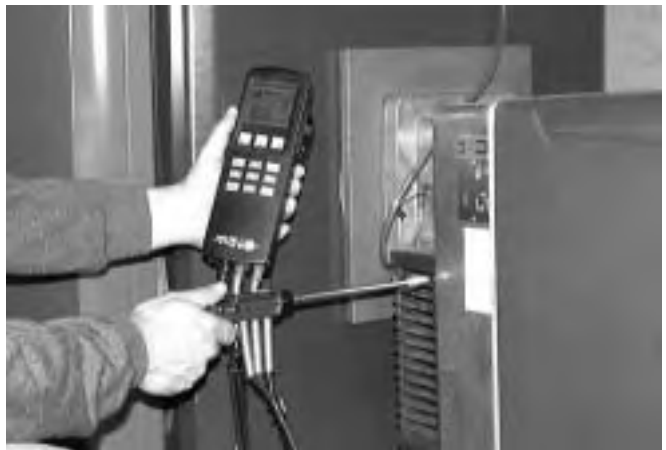
Fig. 12: Measuring the ambient air temperature
