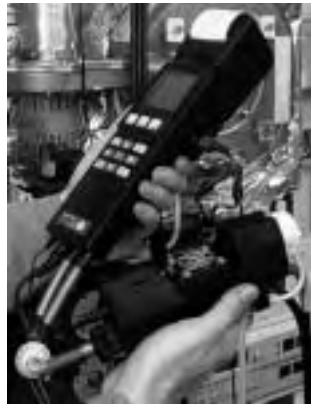
Fig. 19: testo 300 XXL with integrated gas preparation to measure NO 2
