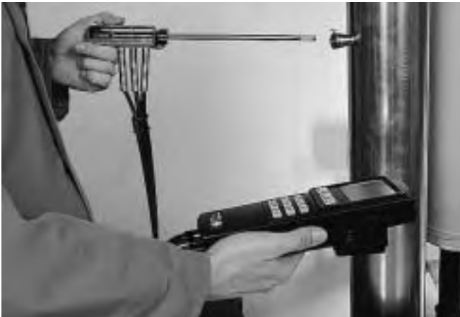
Fig. 13: Determining flue gas loss
