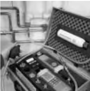
Main test with testo 312-2/3
