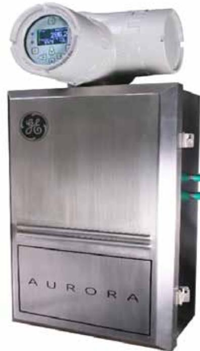
The CO<sub>2</sub> used in this process must be dried to levels of -40°C dew point, about 130 ppmv, or lower. GE's Aurora offers the most reliable and fastest responding moisture analyzer for this application. The analyzer has no wetted moisture sensor and utilized a light energy to instantly measure the moisture content. The Aurora is designed to provide years of operation without user intervention or maintenance.
