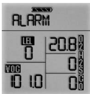
Figure 3-7b. Instrument in VOC Gas Alarm
