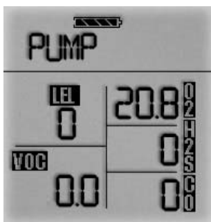
Figure 3-4a. Pump Alarm on the Display
