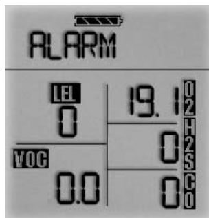
Figure 3-6b. Instrument in Oxygen Alarm
