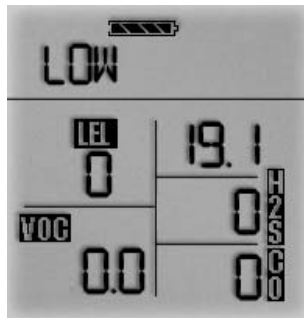
Figure 3-6a. Instrument in Oxygen Alarm
