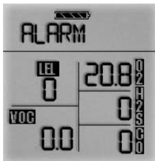
Figure 3-4b. Pump Alarm on the Display
