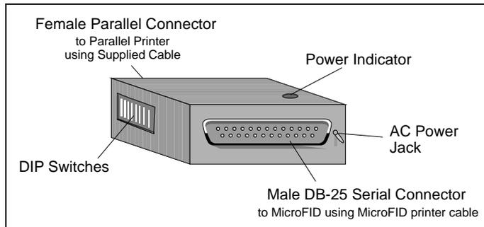
**Figure 19** Serial to Parallel Converter
