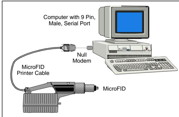
**Figure 25**      **Connecting MicroFID Using the Null Modem Cable**
