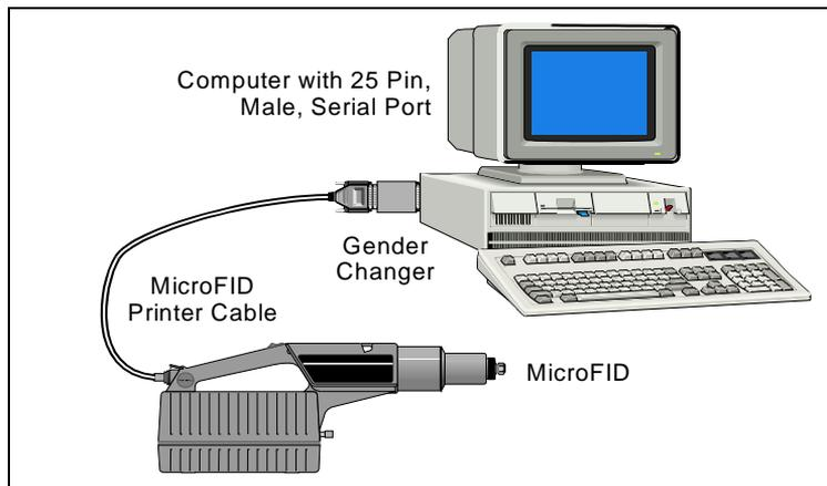
**Figure 26**      **Connecting MicroFID Using the Gender Changer Cable**
