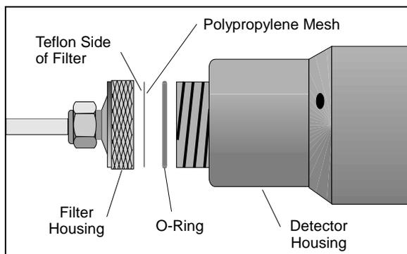
**Figure 23**      **Inlet Filter**
