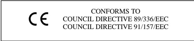
*Council Directive 89/336/EEC - Electromagnetic Compatibility and the Applicable Standards.* MicroFID complies with EN50082-01 Generic Immunity Standard for Electromagnetic Compatibility Part 1: Light Industrial Environment. MicroFID has been tested and conforms to the guidelines specified in EN50082-02 Generic Immunity Standard for Electromagnetic Compatibility Part 2: Industrial Environment
