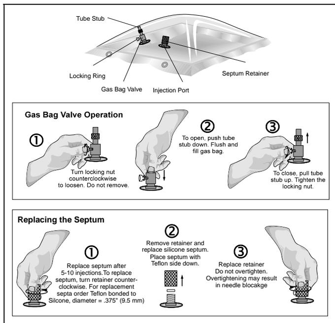
**Figure 11 Using the Gas Bag**
