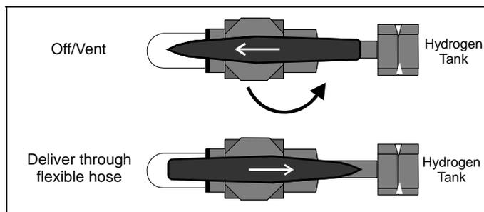
**Figure 3 Refill Adapter 3-Way Valve**
