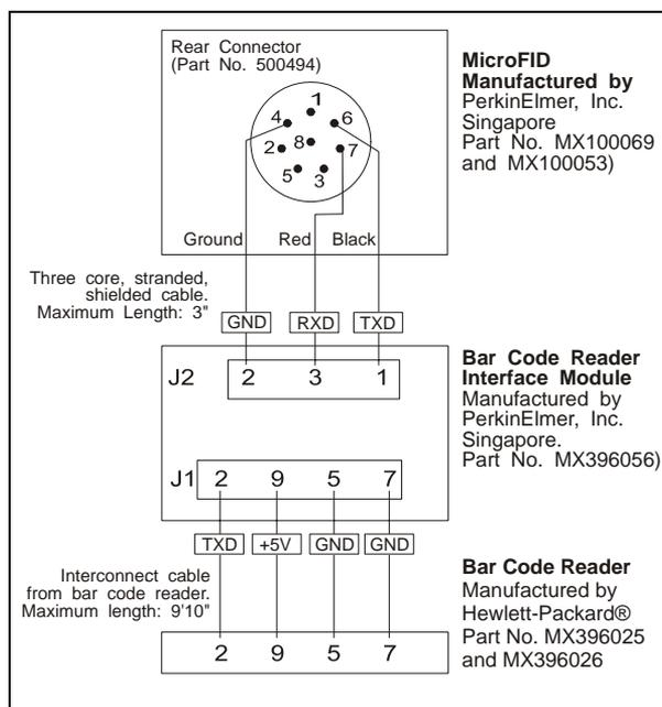
**Figure 29 Bar Code Reader Control Drawing 890047**
