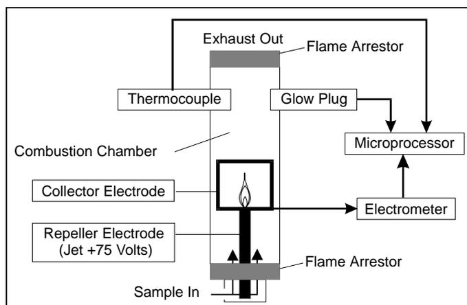
**Figure 27 Flame Ionization Detector**
