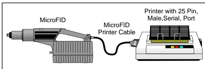
**Figure 12** Connecting MicroFID to a Serial Printer
