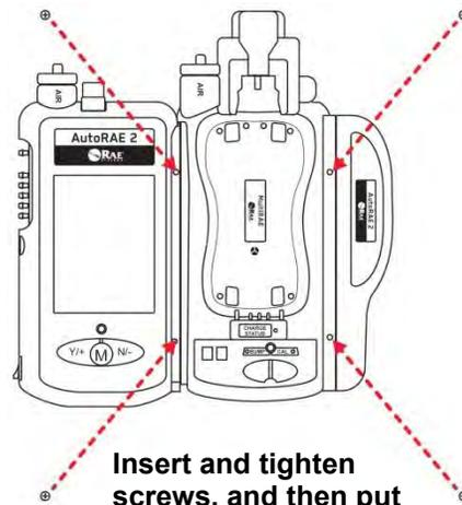
Insert and tighten screws, and then put caps over screws.
