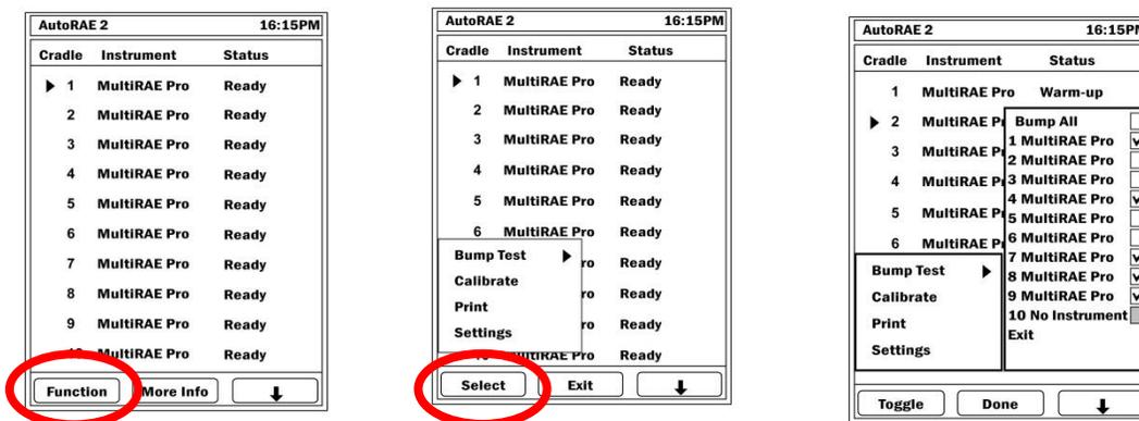
If you did not press [Y/+] to start the process, then a countdown begins. When the countdown reaches zero, then the instruments are bump tested.
