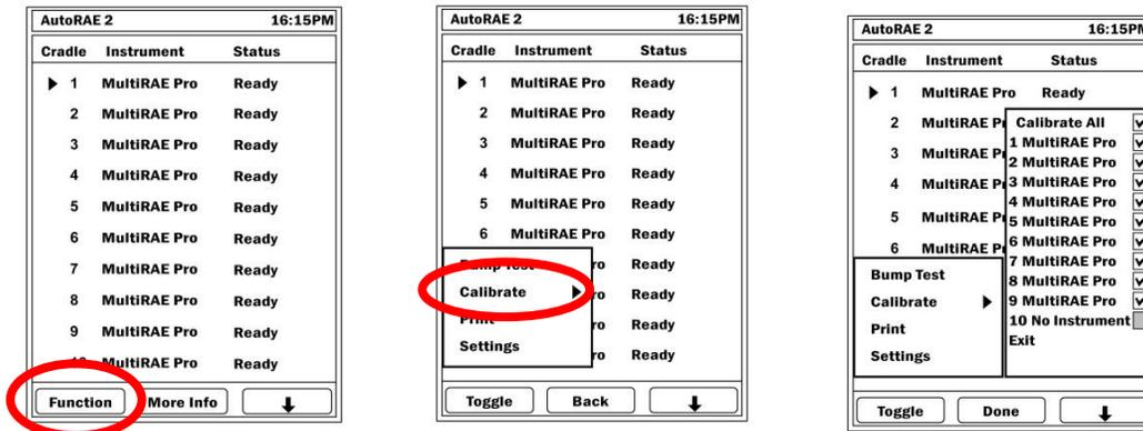
If you did not press [Y/+] to start the process, then a countdown begins. When the countdown reaches zero, then the instruments are calibrated.
