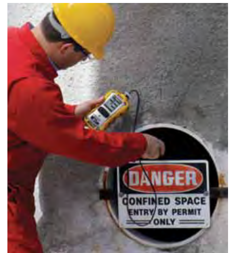
Confined space testing with the MultiRAE Lite
