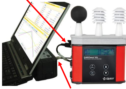
Figure 1-32: Communicating with the QT o 48N and DMS
