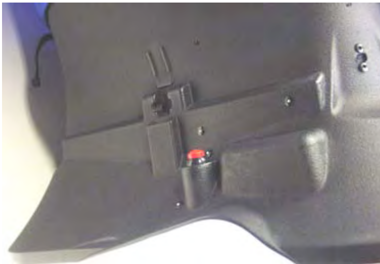
Figure 8 Red Hold Switch Location
