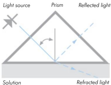
Depending on the angle, some rays are totally reflected. And, some rays are only partially reflected, most of the light is refracted into the process solution.
