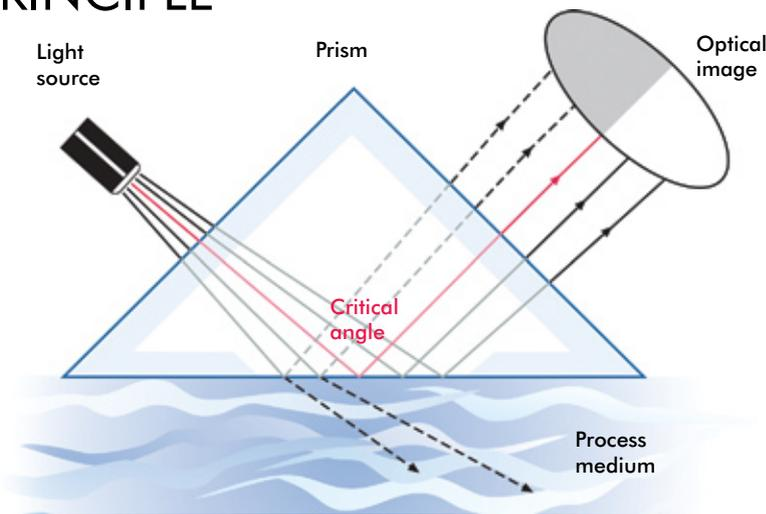
The light source sends light against the interface between a prism and the process solution, where the rays meet the surface at different angles.
