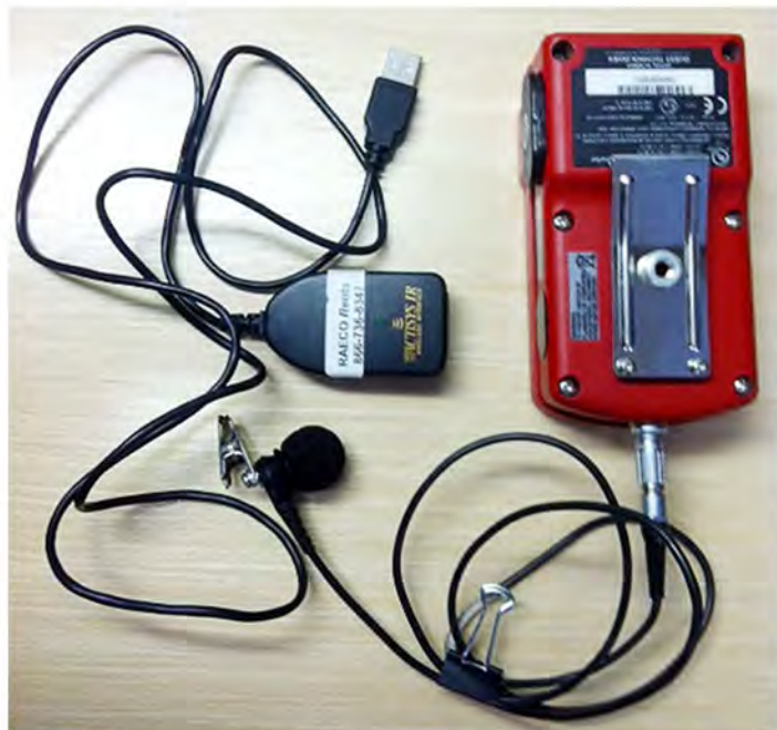
Communicating with a USB port with an infrared cable connection
