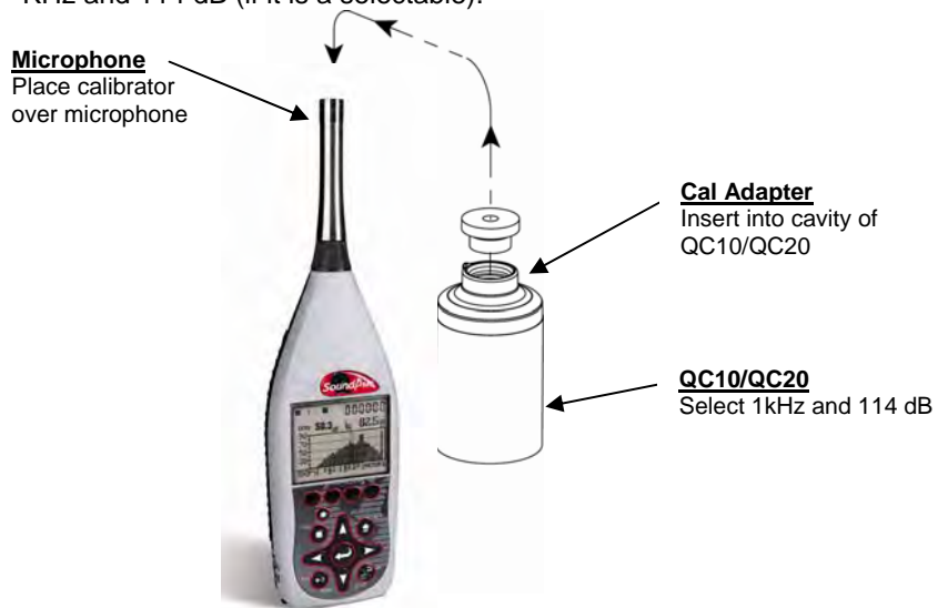
Figure 5-2: Attaching calibrator to the Verifier
