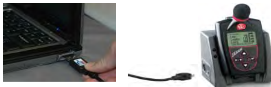
Figure 5-1: Communicating between your pc and the Edge
