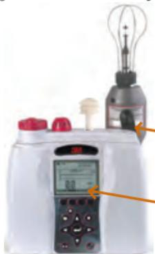
Connect AirProbe to the back housing (two inlets located near the air flow outlet. See air flow diagram on previous page.)
