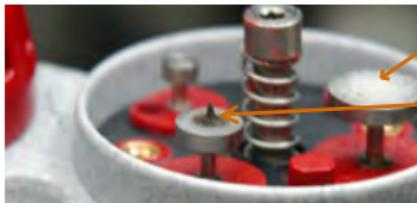
**Thin-layer of silicone** is applied to a clean impactor.
