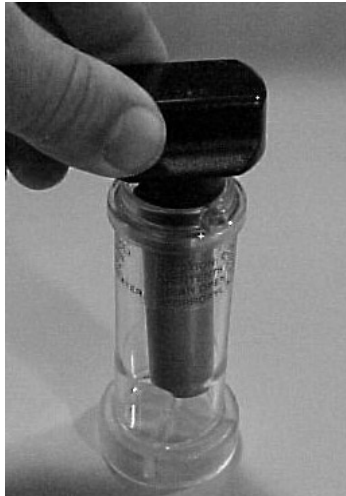
Figure 2-5: Insert Alcohol Cartridge into Fill Capsule
