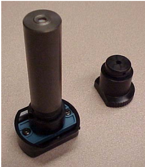
Figure 2-3: Alcohol Cartridge and Storage Cap
