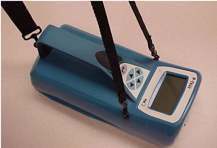
Figure 2-9: Attach Shoulder Strap to Instrument
