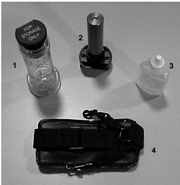
Figure 1-2: Alcohol Fill Capsule with Storage Cap, Alcohol Cartridge, Alcohol Bottles and Shoulder Strap
