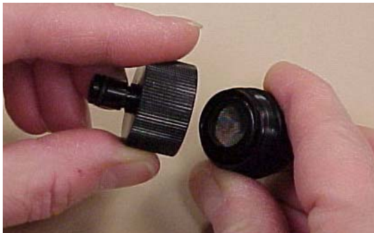
Figure 4-4: Re-assemble Inlet Screen Assembly
