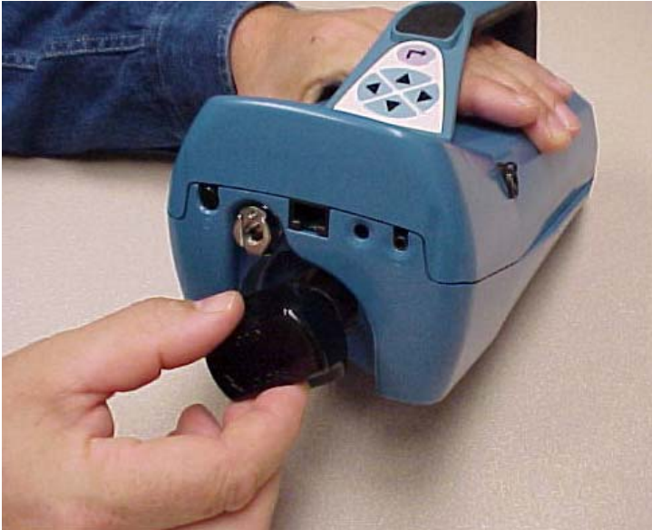
Figure 2-6: Insert Alcohol Cartridge into P-TRAK
