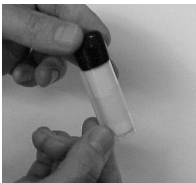
Figure 4-2: Remove Wick and Screen Using Dowel
