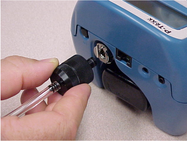
Figure 2-7: Insert Inlet Screen Assembly into Fitting
