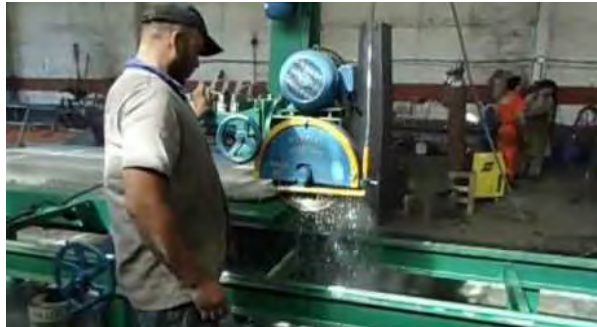
A worker cutting granite using a saw that applies water to the blade. The water reduces the amount of silica-containing dust that gets into the air.
